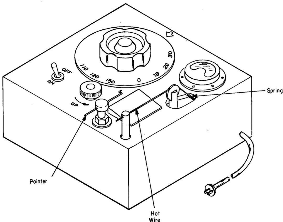
Short sections of glass tubing can be split accurately so that the cuts are aligned 180° apart. A heated wire is incorporated with a positioning mechanism to make the cuts along the major axis of the tube. The re-assembled tube forms a low-pressure, gastight enclosure.
