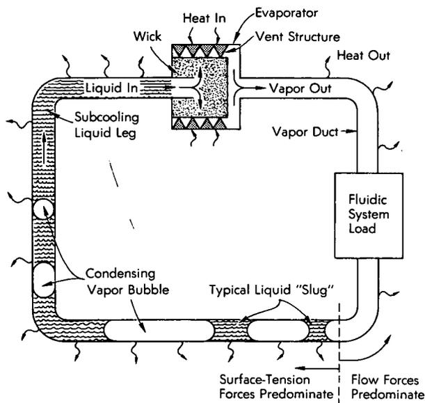
dynamic properties for circulation in a capillary-pumped heat transfer loop. The fluid is vaporized in an evaporator, passed through a fluidic system load, condensed, pumped by a multistage capillary pump, and returned to the evaporator. Condensate pumping is provided by the capillary pumps of the form that are used extensively for heat-transfer applications.
