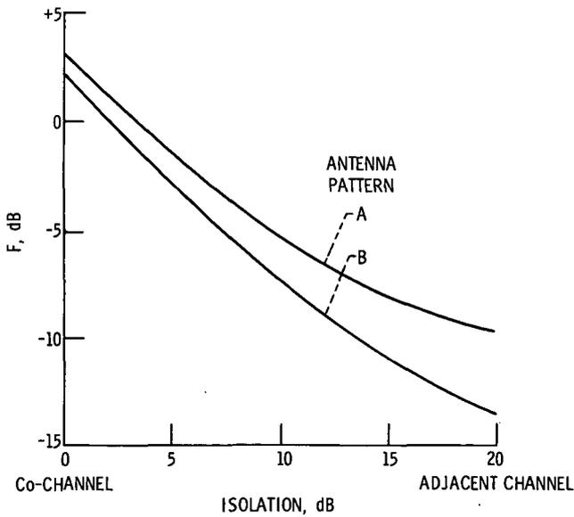
Figure 12. - Factor "F" as a function of channel isolation for the two antenna side lobe patterns shown in figure 2. Receiving antenna pattern A,  $N = 2.5$ ,  $P_C/P_D = 0$  dB, separate grouping, single satellite sharing.
