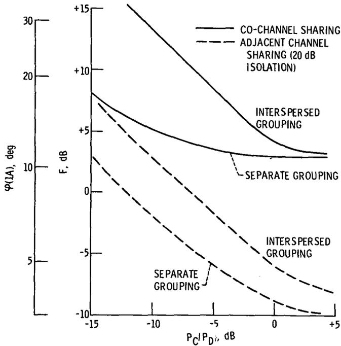
Figure 8. - Factor F and  $\varphi$  as a function of satellite power ratio  $P_C/P_D$  for two grouping schemes and two frequency divisions, receiving antenna pattern A,  $N = 2.5$ . For the determination of  $\varphi$ , receiver system 1A was used.
