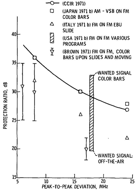
Figure 2. - FM - Television Protection Ratio for weighted signal-to-noise ratios greater than 49 dB.
