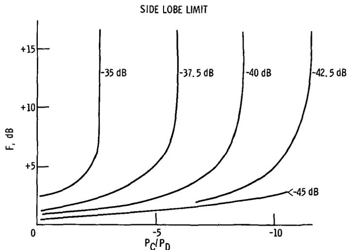
Figure 7. - Spacing factor  $F$  as a function of  $P_C/P_D$  and receiving antenna for side lobe limit.  $P_R = 30$  dB, receiving antenna pattern "A", separate grouping, one typical receiver location.
