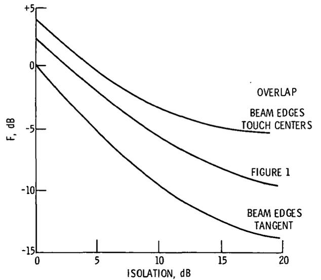
Figure 13. - Orbit Spacing Factor, F, as a function of channel isolation and degree of pattern overlap,  $P_C/P_D = 0$  dB, receiving antenna pattern A,  $N = 2.5$ , separate grouping, single satellite sharing.
