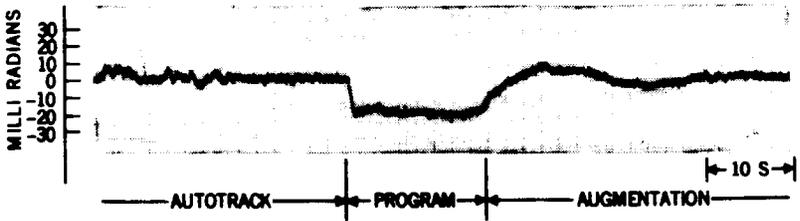
Figure 3—Configuration of the tracking loop with augmentation added and the response of this loop (tracking error versus time).
