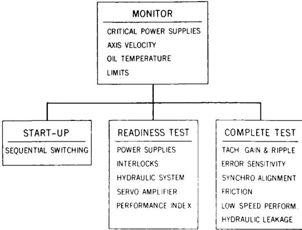
Figure 1—Program for the monitoring and automatic checkout of the antenna servo system.
