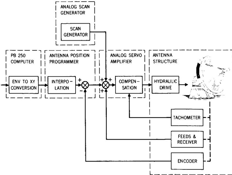
Figure 2—Tracking loop for a typical STADAN antenna.
