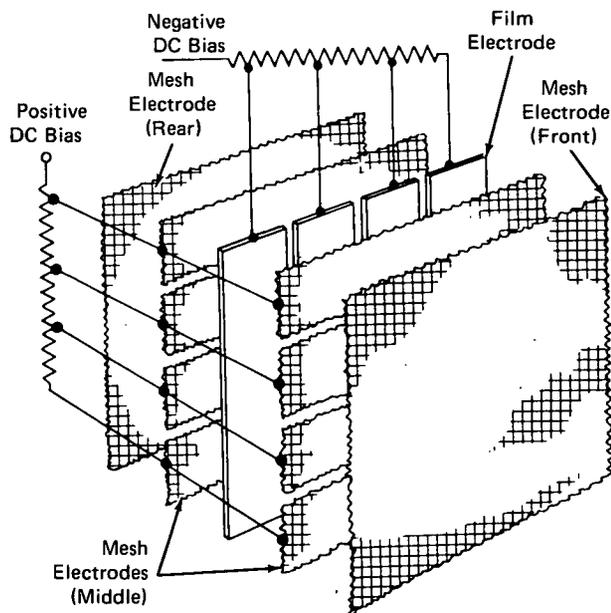
Figure 1. Particle Detector Showing the Five Planar Electrodes
