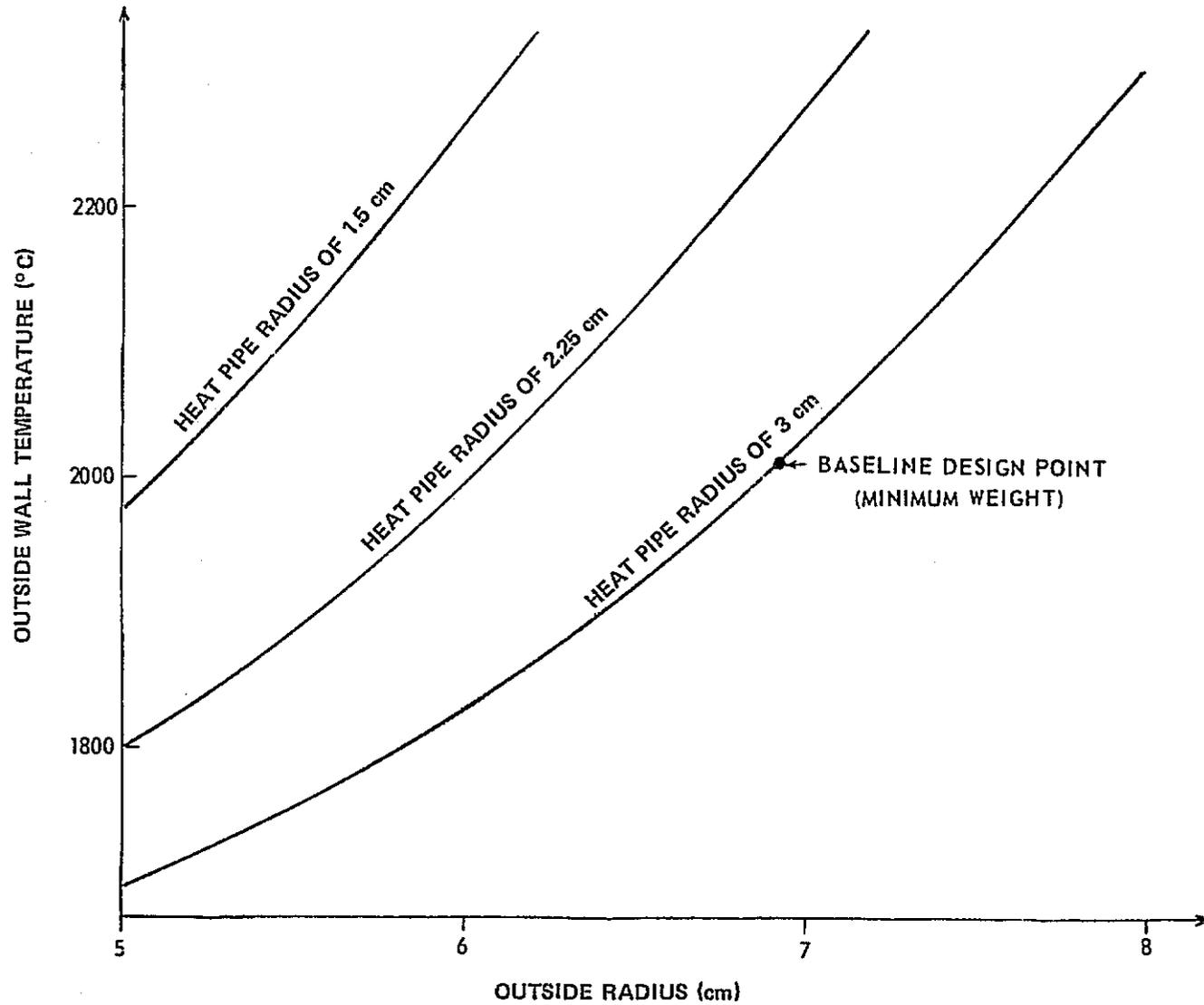
Figure 23. Outside temperature of actinide cylinder versus radius of cylinder (inside temperature of 1600°C).
