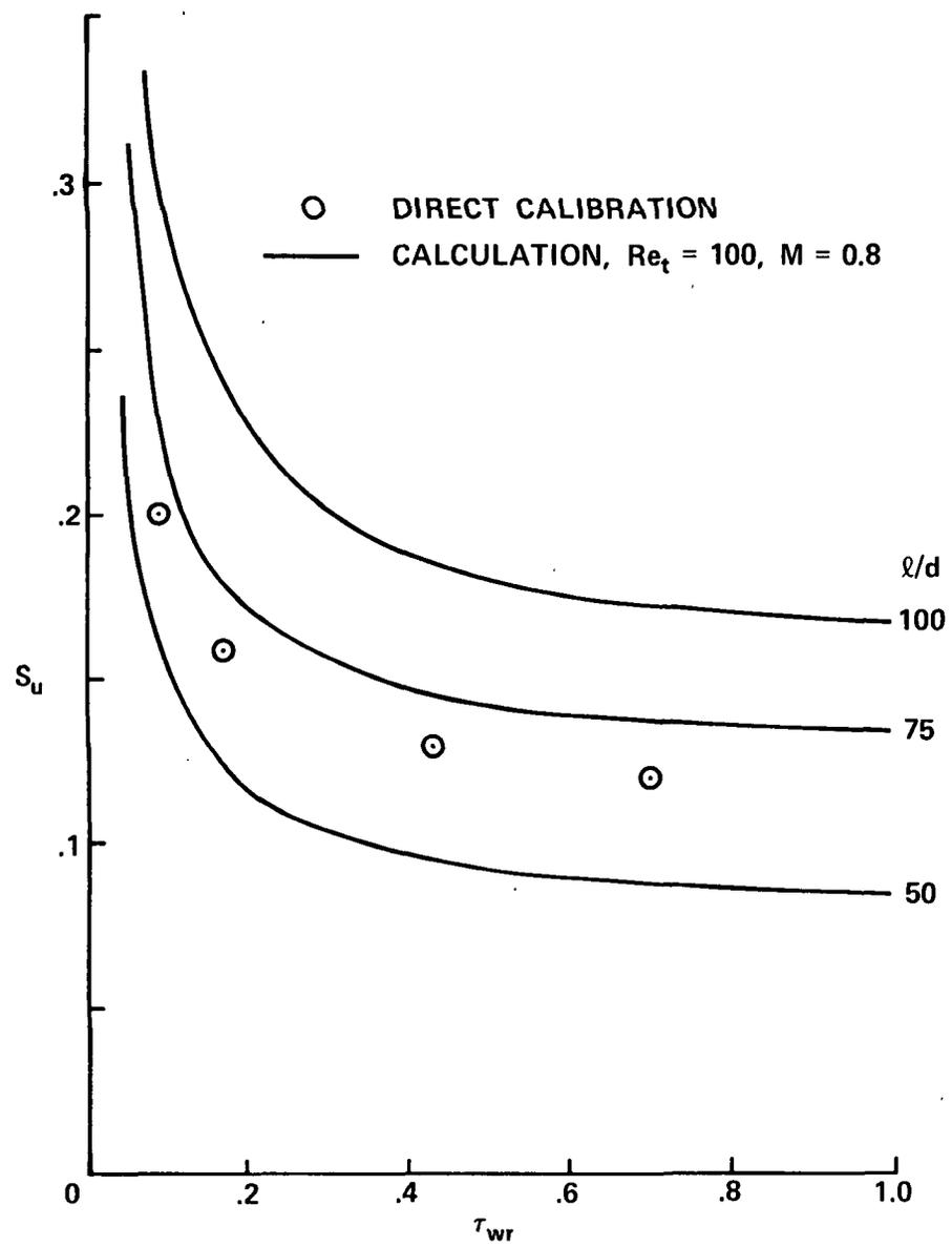
Fig. 2. Comparison of calculated and measured velocity sensitivities.
