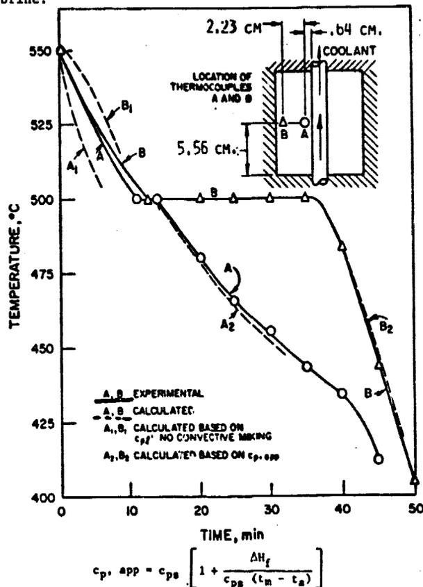
Fig. 6 - Cooling rates in a lab-scale thermal energy storage unit
