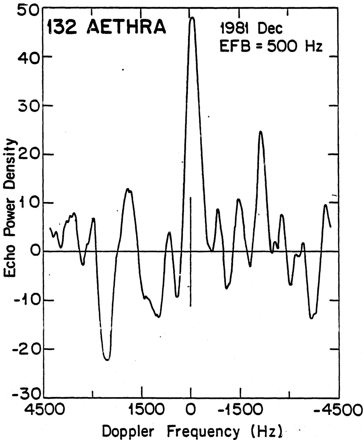
detection and if Aethra's radar reflectivity is close to the asteroidal average, then this object's diameter is somewhat larger than 100 km, and its rotation period is less than 10 hours. Neither Kalliope nor Papagena were detected.
