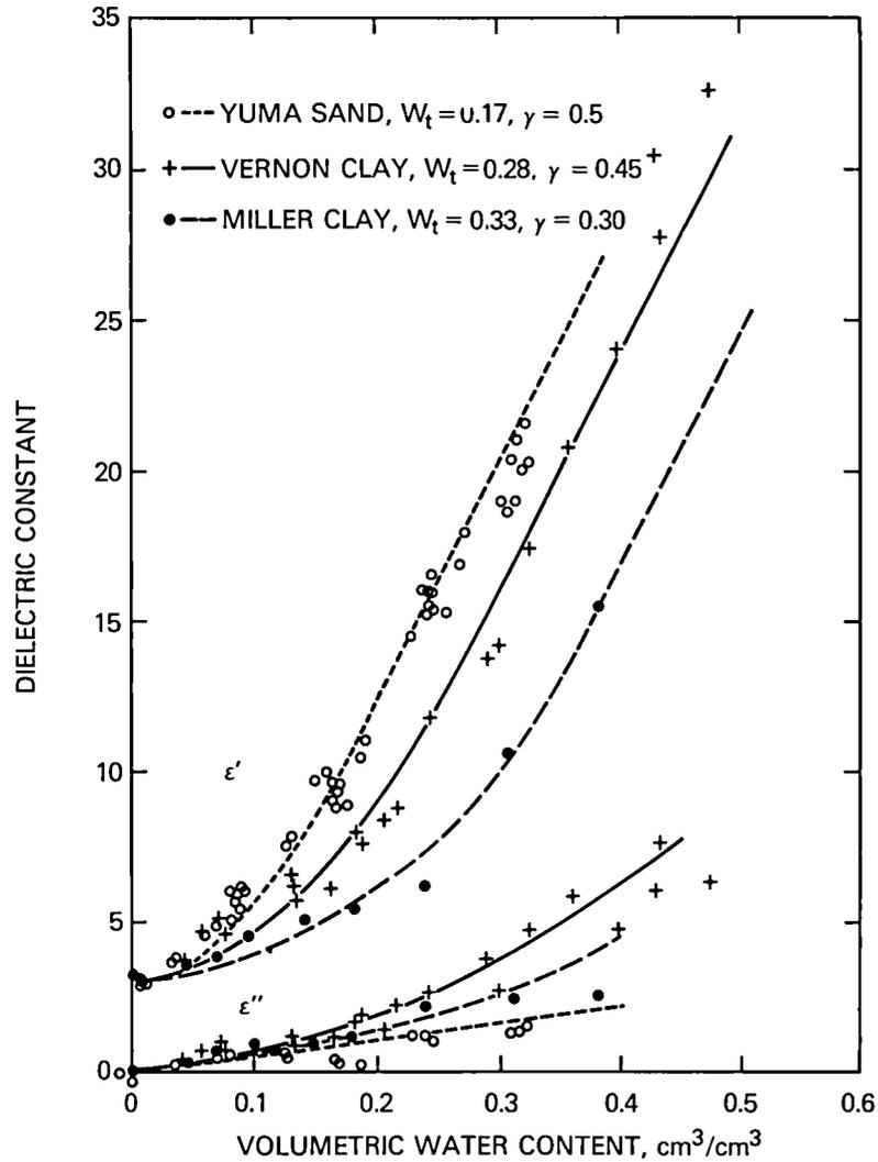
Figure 1. Laboratory measurements of the real and imaginary parts of the dielectric constant for 3 soils at a wavelength of 21 cm.
