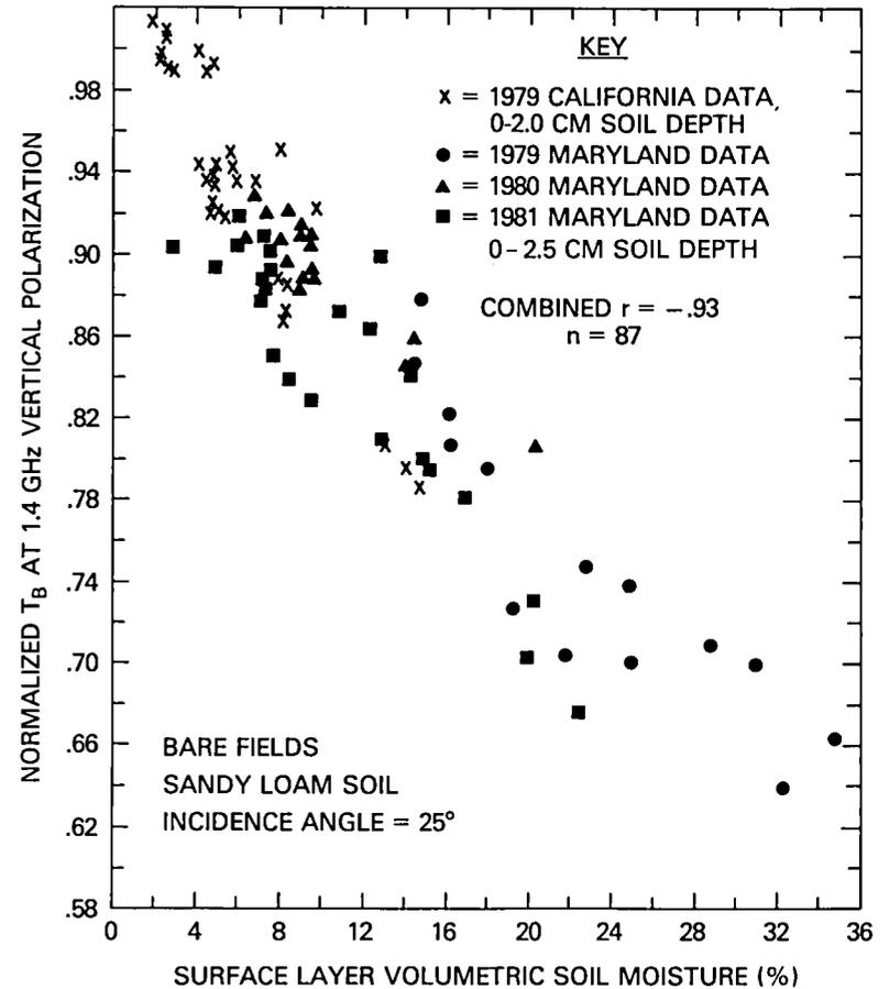
Figure 2. Observations of microwave emissivity from a tower.
