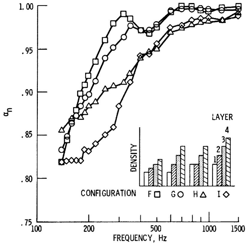
Figure 11. - Measured normal absorption coefficients of 4 layer configurations.
