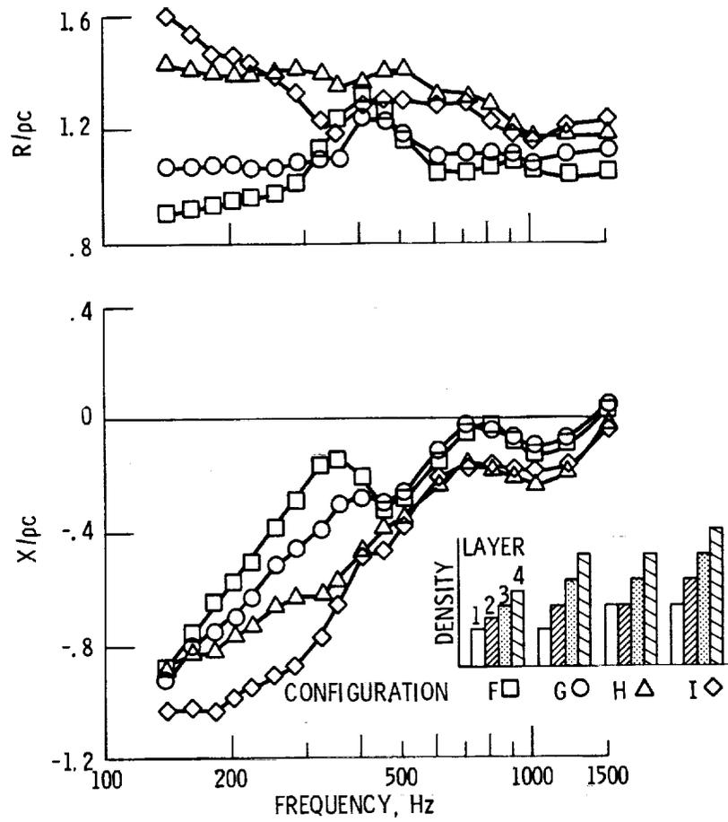
Figure 10. - Measured specific acoustic impedance of 4 layer configurations.
