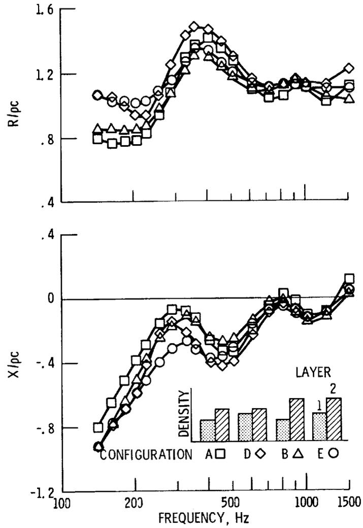
Figure 8. - Measured specific acoustic impedance of 2 layer configurations with variations in the first layer density.
