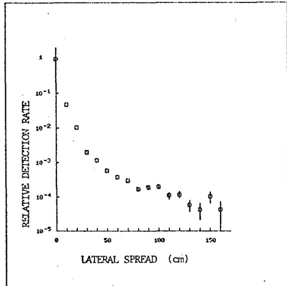
Figure 4. Relative detection rate versus lateral particle spread.
