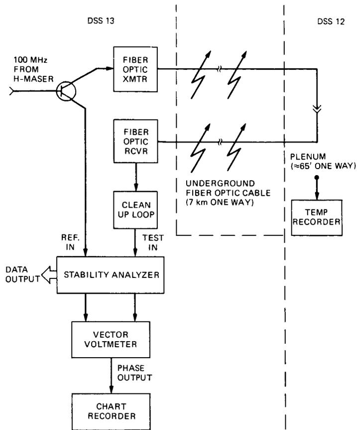
Fig. 6. Simplified block diagram of the test set-up
