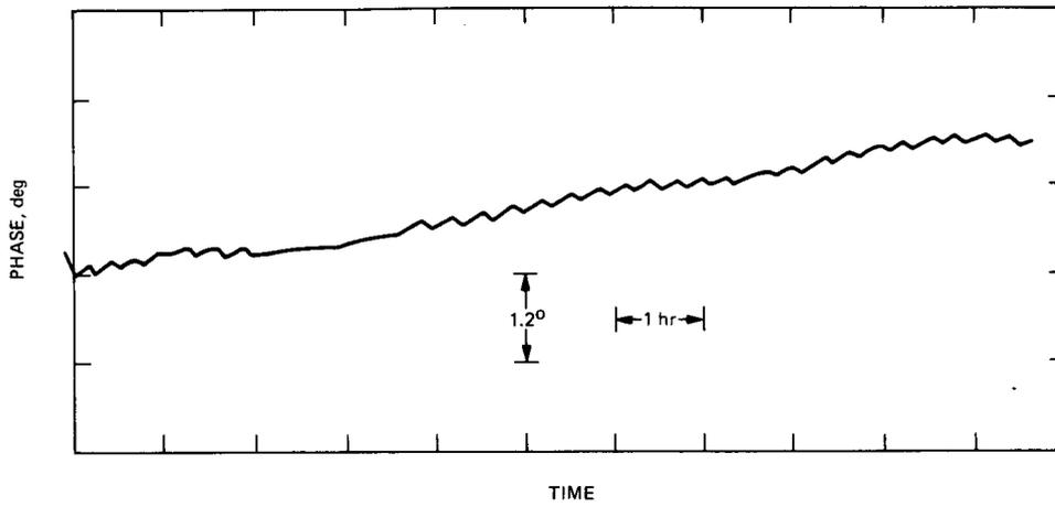
**Fig. 4. Phase measured across the fiber-optic link**
