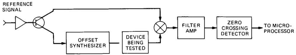
**Fig. 3. Simplified block diagram of the stability analyzer**
