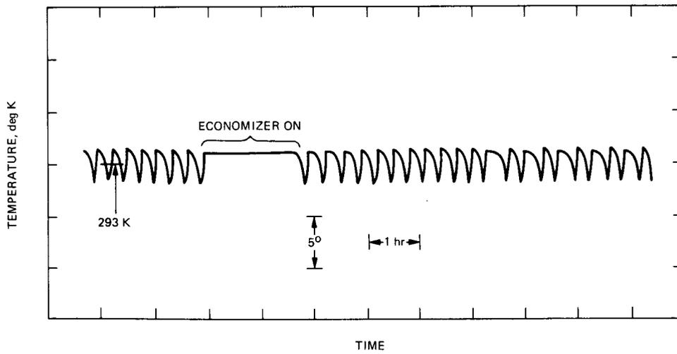
**Fig. 5. Temperature measured in the Echo station plenum**
