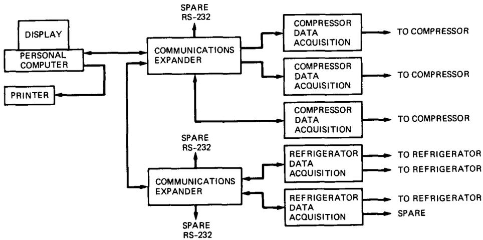
Fig. 3. CCR data acquisition system block diagram
