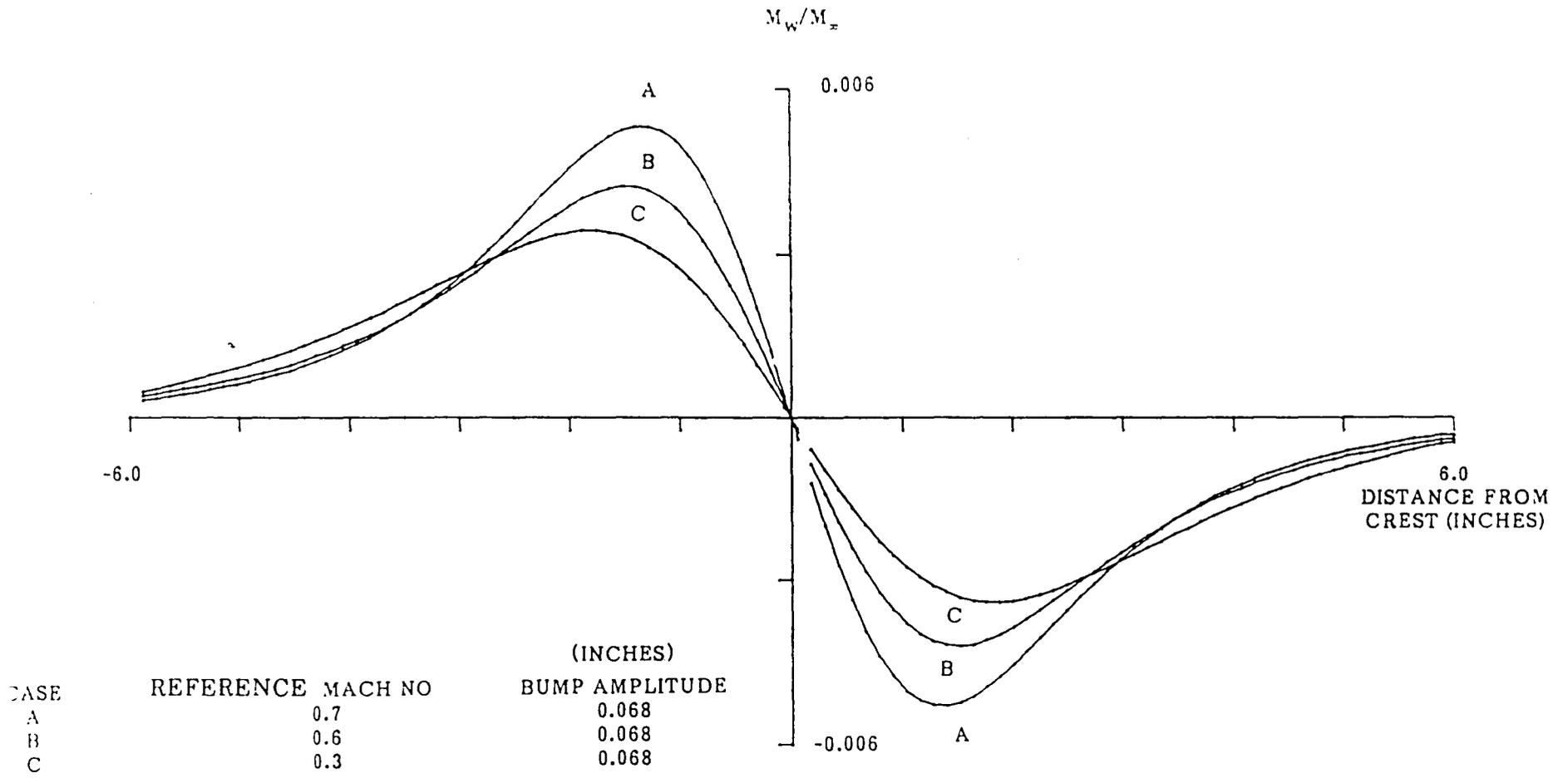
**FIGURE 2** THEORETICAL W-PERTURBATIONS (INCLUDING BOUNDARY LAYER EFFECTS)
