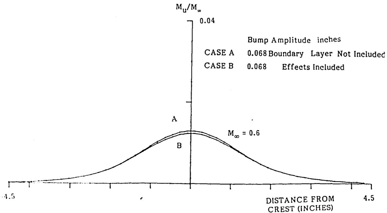
FIGURE 10 THEORETICAL U-PERTURBATIONS VS DISTANCE FROM BUMP CREST
