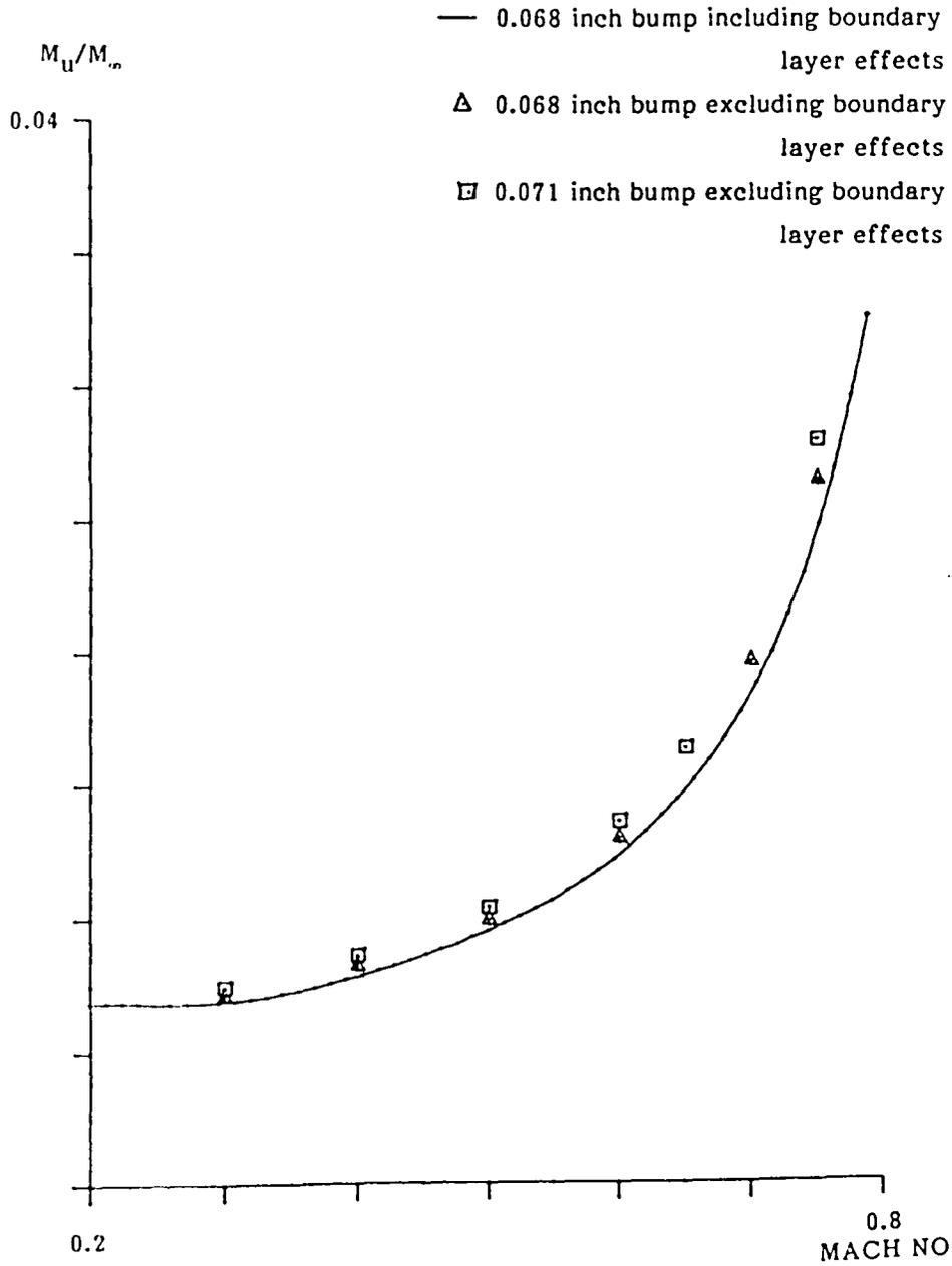
FIGURE 11 : THEORETICAL ESTIMATES OF THE EFFECT OF MACH NUMBER AT THE U-PERTURBATION AT THE TUNNEL CENTRELINE IN LINE WITH THE BUMP CREST
