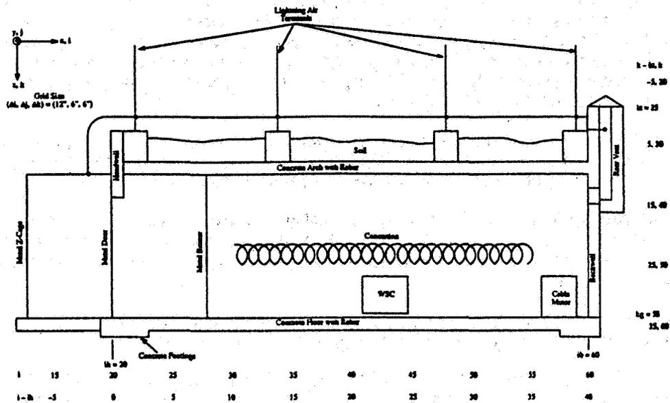
Figure 4 Igloo Vertical Cross-Section at  $j = j_m = 75$
