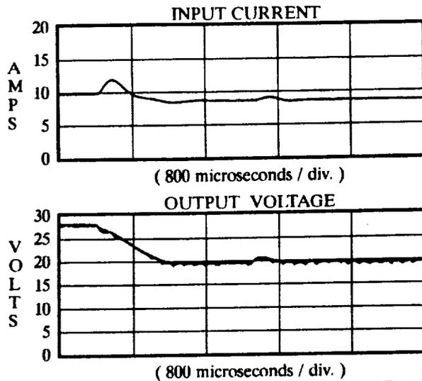
Figure 6. Zero Voltage Switching Converter Overload Test
