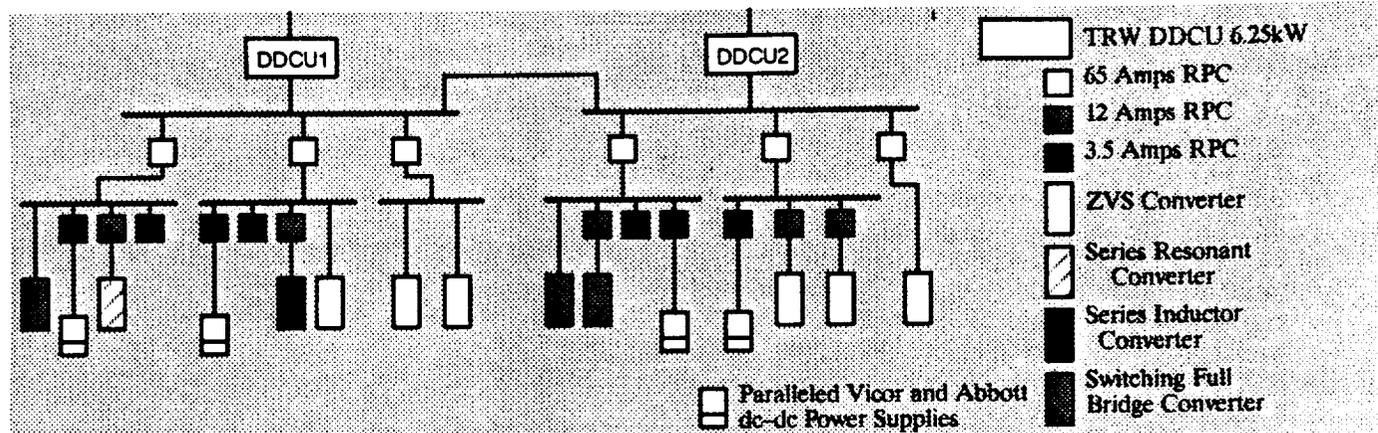
Figure 2. PMAD DC Test Bed Secondary System Configuration
