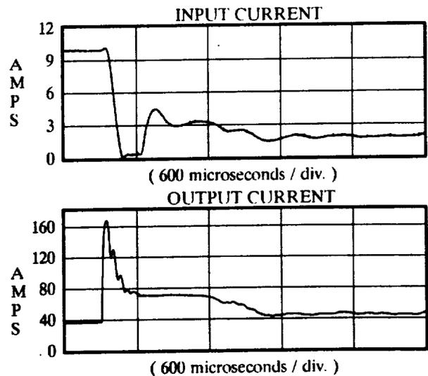
Figure 8. Series Resonant Converter Short Circuit Test
