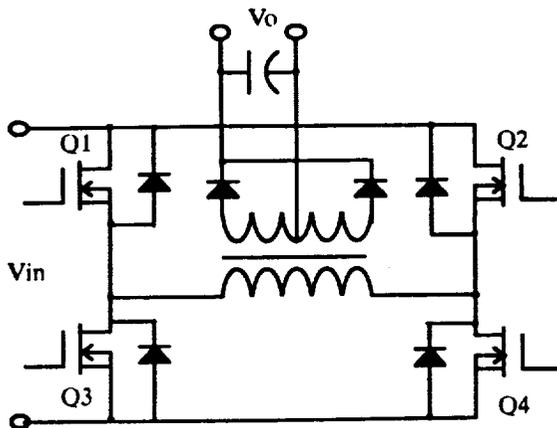
Figure 1. Zero Voltage Switching Topology Power Stage
