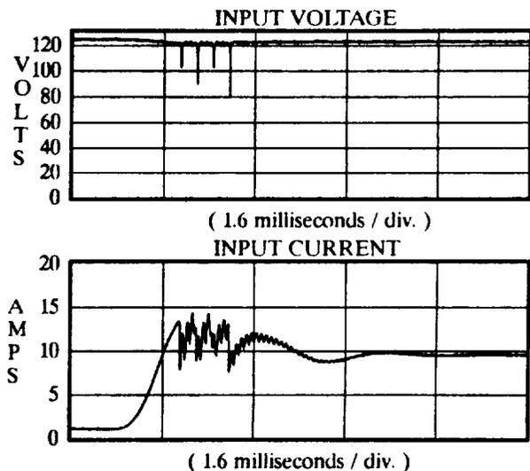
Figure 5. Switching Full Bridge Converter Load Step Test
