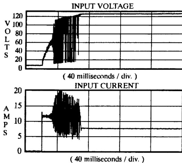
Figure 4. Switching Full Bridge Converter Inrush Test
