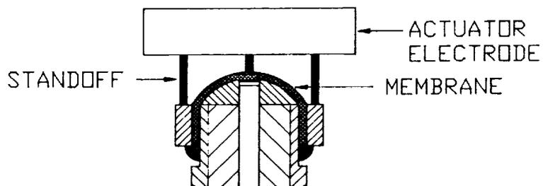
FIGURE 1. ELECTROSTATIC ACTUATOR FOR HIGH TEMPERATURE MICROPHONE CALIBRATION.
