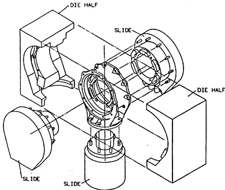
Figure 4. Conceptual Drawing of Outer Housing Die Assembly
