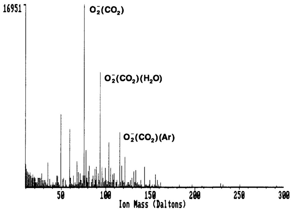
**Figure 6. Negative Reactant Ions Using Argon for the Carrier and Drift Gases and  $CO_2$  for the Sample Gas.** 1.1% Purified Air (bottom) and 6.3% Purified Air (top) was introduced into the Argon Drift Gas.
