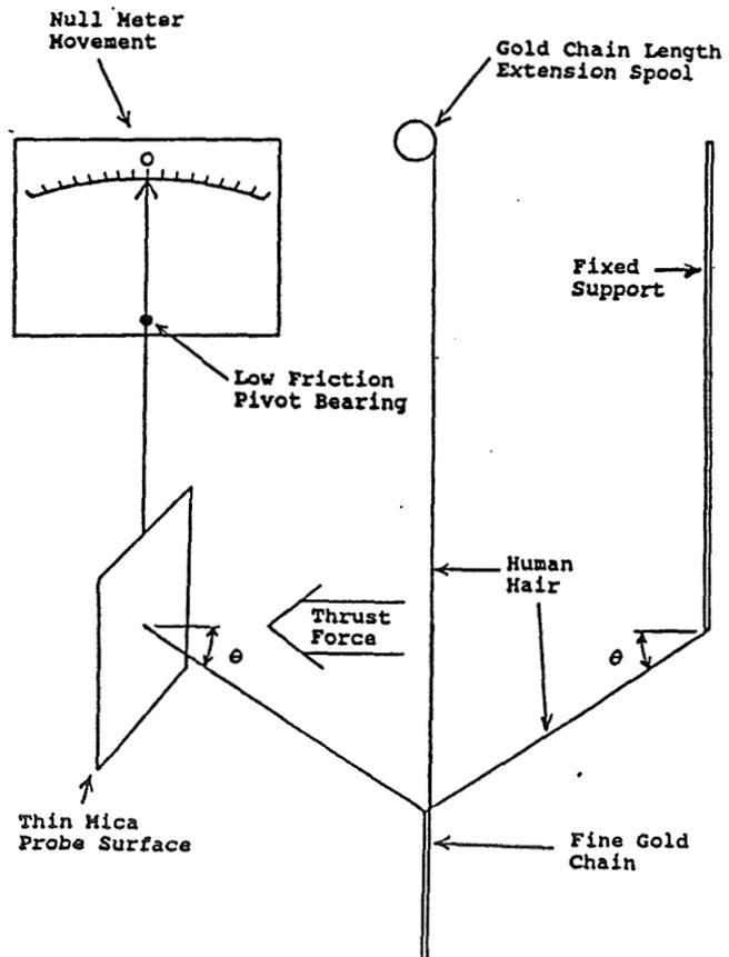
Fig. 4 Primary components of the momentum probe.
