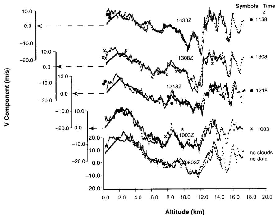
Fig. 2 Five  $v$  wind components of the NASA 50-MHz Radar Wind Profiler (data) overlaid on the wind profile of FPS-16 Radar/Jimsphere (solid line) measured during the STS-37 launch, April 5, 1991, at KSC, Florida. Symbols  $x$  and  $o$  indicate GOES-7 Satellite wind data.
