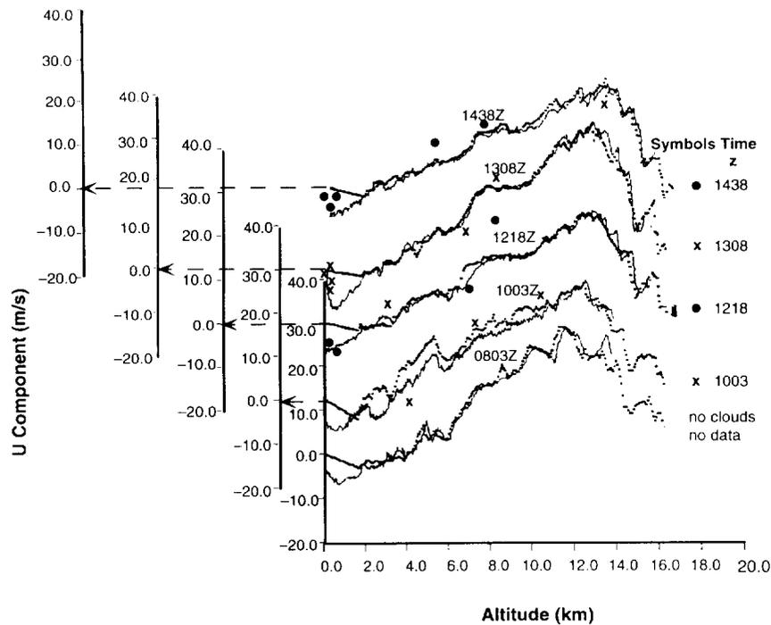
Fig. 1 Five  $u$  wind components of the NASA 50-MHz Radar Wind Profiler (data) overlaid on the wind profile of FPS-16 Radar/Jimsphere (solid lines) measured during the STS-37 launch, April 5, 1991, at KSC, Florida. Symbols  $x$  and  $o$  indicate GOES-7 Satellite wind data.
