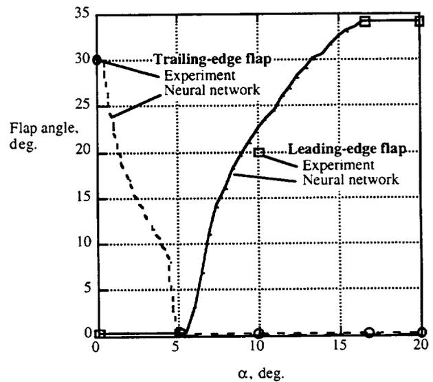
Figure 14. Flap schedule generated using neural-network model which maximizes L/D across angle-of-attack range from 0° to 20°.
