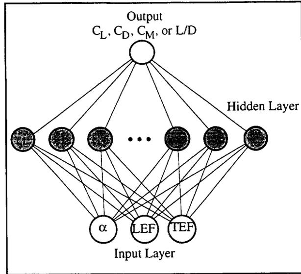
Figure 3. Neural-network architecture used for modeling aerodynamics.
