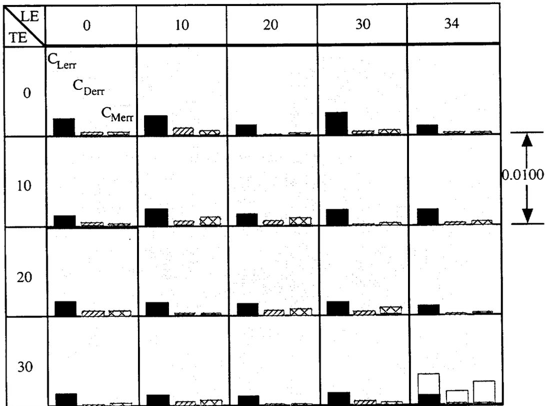
Errors for LEF/TEF = 15°/10°:  $C_{Lerr} = 0.0020$ ,  $C_{Derr} = 0.0002$ ,  $C_{Merr} = 0.0003$ .
