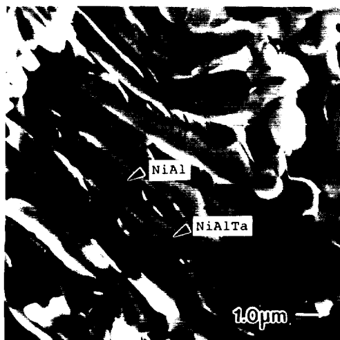
Fig. 9. SEM photomicrographs of fracture surfaces from a NiAl-14.5Ta bend specimen.
