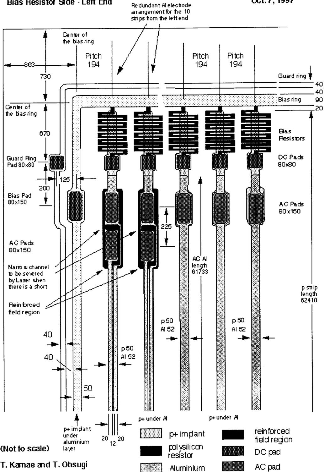
Figure 2: Silicon Strip Detector for the GLAST Prototype Tower. The linear dimension is in  $\mu\text{m}$ .
