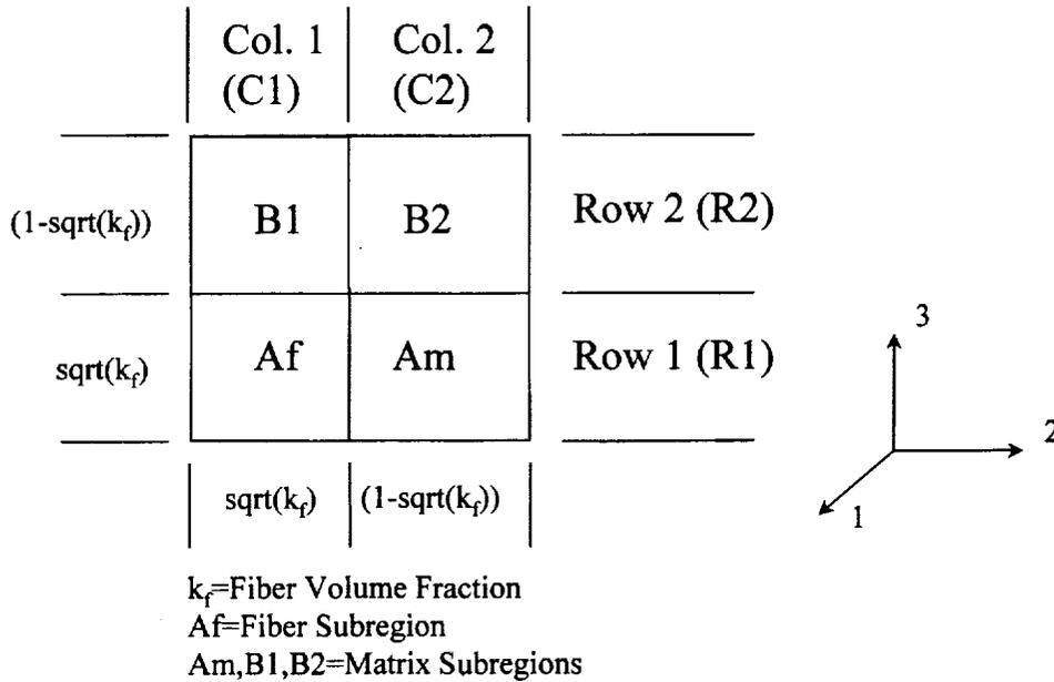
Figure 2: Geometry and Layout of Unit Cell Model.
