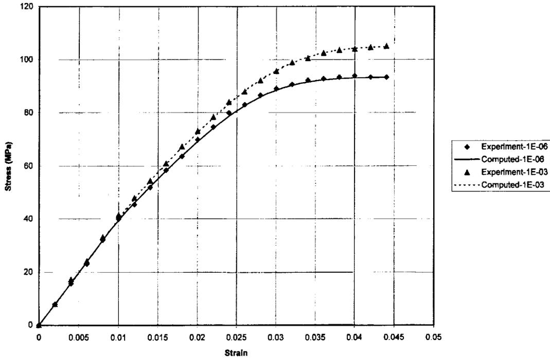
Figure 1: Model Correlations of PEEK Thermoplastic at Strain Rates of  $1 \times 10^{-6}$ /sec (1E-06) and  $1 \times 10^{-3}$ /sec (1E-03).
