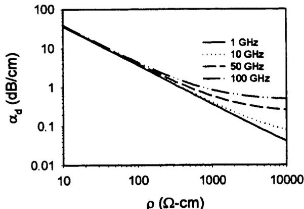
Fig. 1: Calculated dielectric attenuation of 50  $\Omega$  microstrip line on 100  $\mu\text{m}$  thick Si and a line width of 80  $\mu\text{m}$ .
