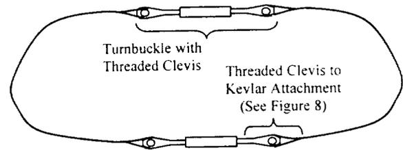
Figure 7: Kevlar Cable Assembly with Turnbuckle
