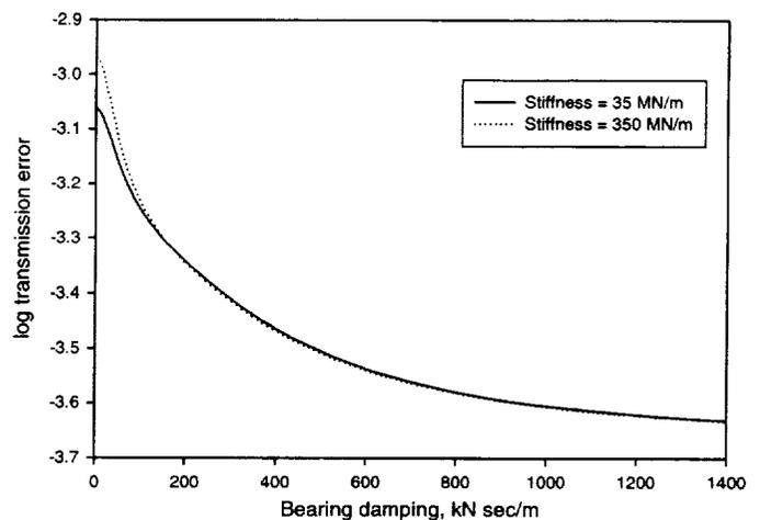
Figure 3. Dynamic transmission error at twice mesh frequency; shaft speed, 114 Hz.
