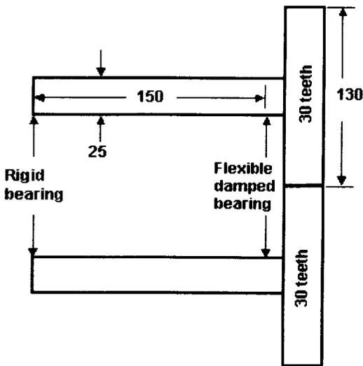
Figure 1. Gear system model (dimensions in mm).
