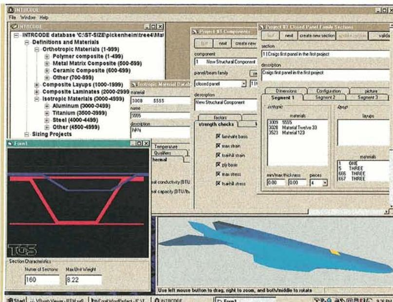
*Collier R&D’s HyperSizer software, developed from NASA technology, displays an aircraft’s surface in multicolored pixels.*
