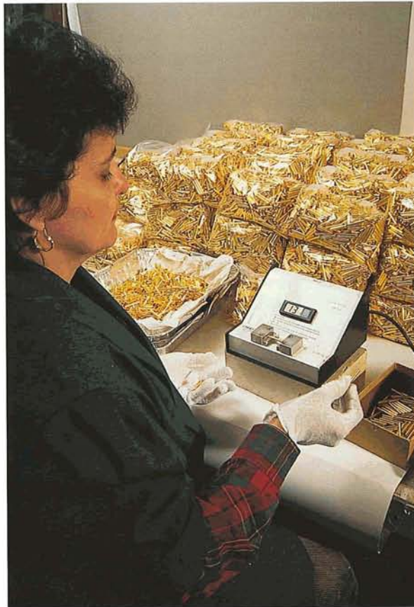
Each Laser Gold-coated tube used for the tympanic thermometer is inspected for reflectivity and dimensions by hand.
