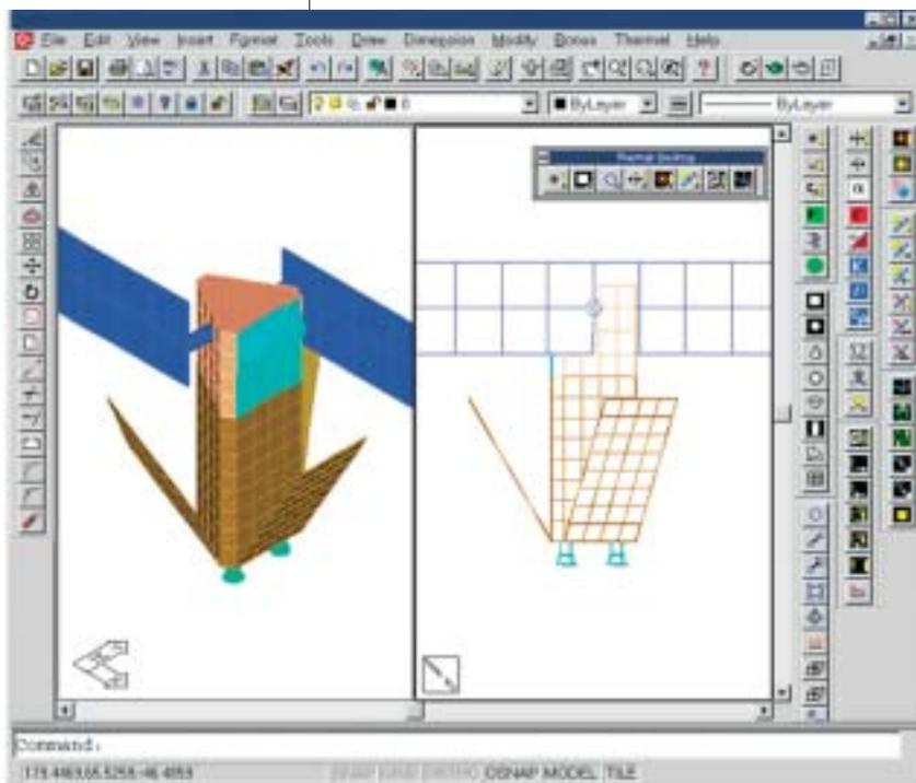
completed the development of *SinapsPlus*,<sup>®</sup> which also originated from the founders of C&R while at Martin Marietta. *SinapsPlus*, a sketchpad graphical user interface (GUI), provides a visual means of accessing the solution power of SINDA/FLUINT, making the system more approachable.
