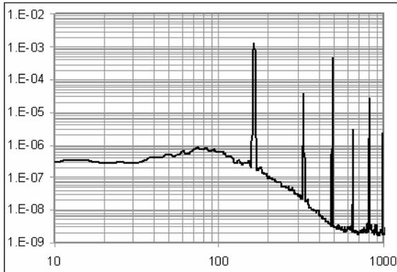
Figure 10. HSS Radial Bearing Position Spectrum
