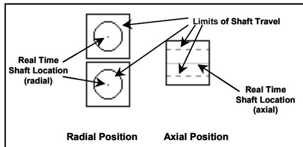
Figure 3. MB Operator Console – Shaft Position
