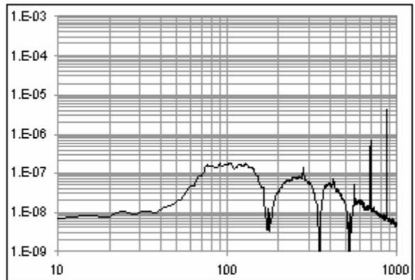
Figure 11. HSS Radial Bearing Current Spectrum
