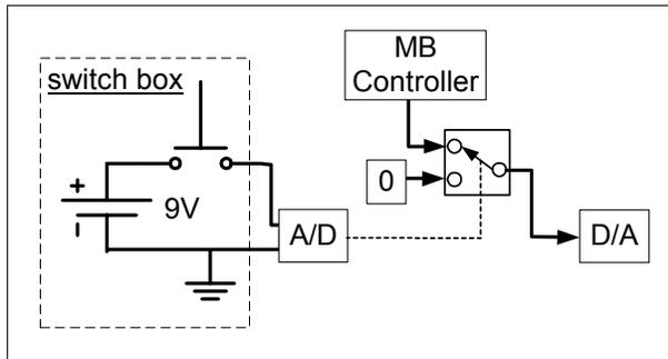
Figure 18. Bearing Current Zeroing Implementation
