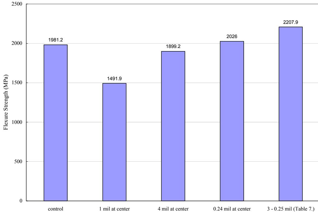
Figure 4.2. Flexural strengths of Al-Mylar™ Interleaf IM-7/977-3 Composites.
