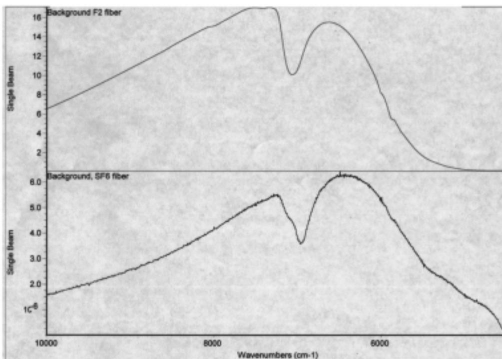
**Figure 4. Single beam spectra of F2 and SF6 optical fibers
