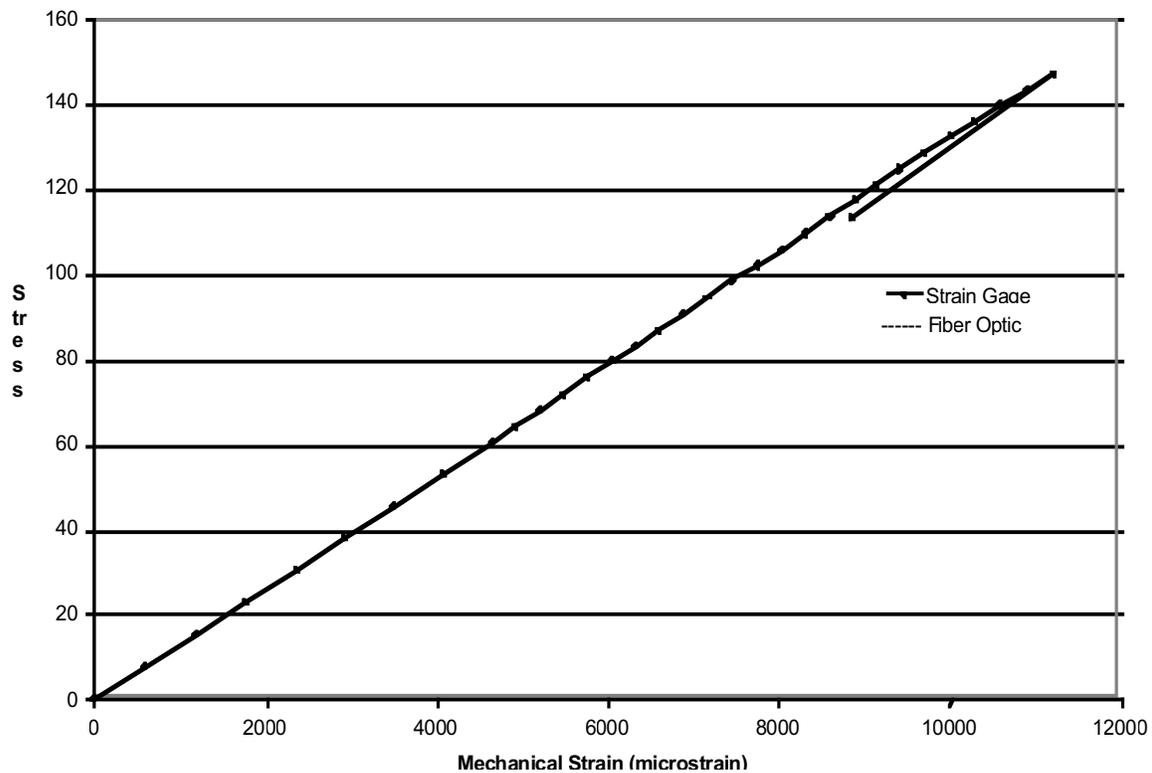
**Figure 8. Tensile specimen #1 high strain level results**
