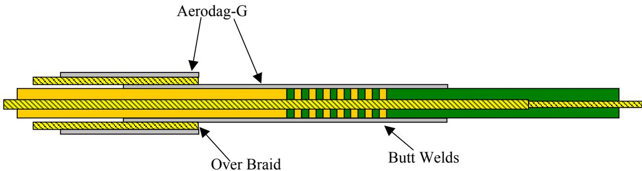
**Figure 7. ProSEDS Tether Triple Point Mitigation Design**
