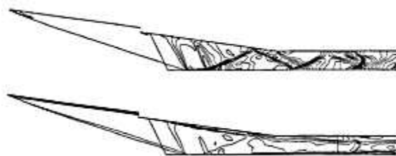
Subscale inlet pressure ( p/p_{\infty} ) and Mach number contours for a supercritical flow of M_{\infty} = 5 . Top: pressure contour ranges of 1.4 to 32.2. Bottom: Mach number contour ranges of 0.2 to 5.0.
