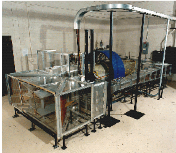
Scale Model Icing Research Tunnel (SMIRT).
