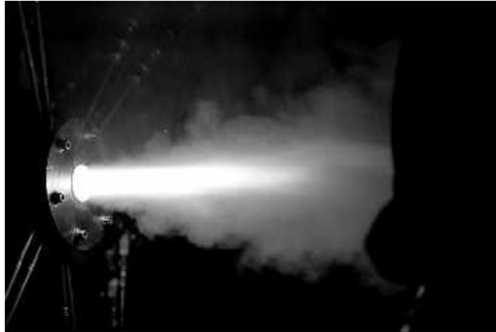
*Gelled propellant engine test: 55-wt % RP-1/Al.*
