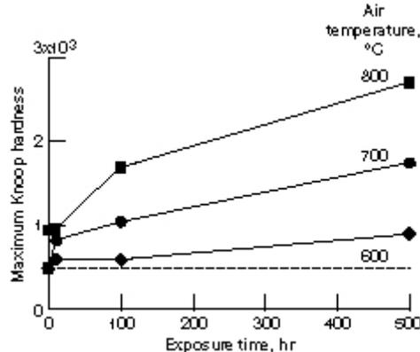
*Near surface hardening of O-Ti as a function of air exposure duration at 600, 700, and 800 °C. The horizontal dashed line indicates the baseline hardness of the unexposed material.*
