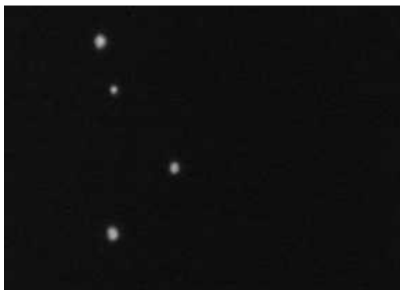
Flame balls from a mixture of 4 vol % hydrogen in air, 30 sec after ignition. The flame ball diameters ranged from 5 to 15 mm.
