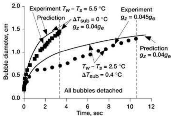
*Comparisons of measured bubble diameter and numerical prediction in saturated water and in subcooled water at low gravity. Time,  $t$ , 0 sec; wall superheat,  $DT_{sub}$ , 0.3 °C; wall temperature minus the saturated liquid temperature,  $T_w - T_s$ , 4.2 °C; Earth's gravitational acceleration in the z-direction,  $g_z \gg 0.02 g/g_e$  (where  $g_e$  is Earth's normal gravitational acceleration).*
