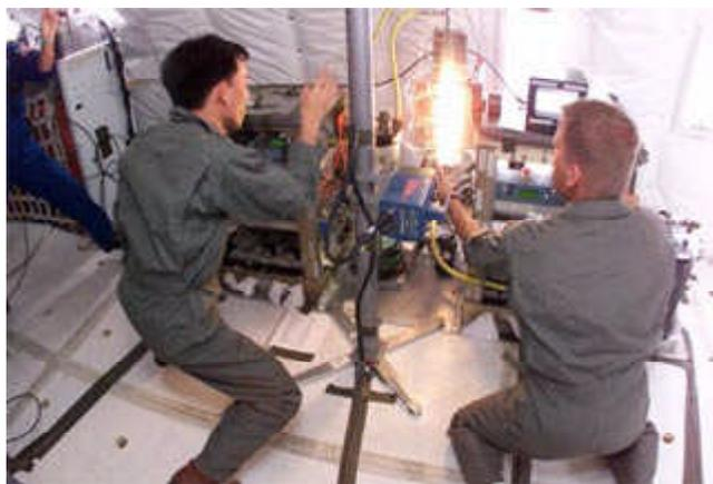
*Researchers Eric Dao (University of Houston) and Brian Motil (Glenn) work on a packed bed reactor experiment on NASA's KC-135 aircraft.*
