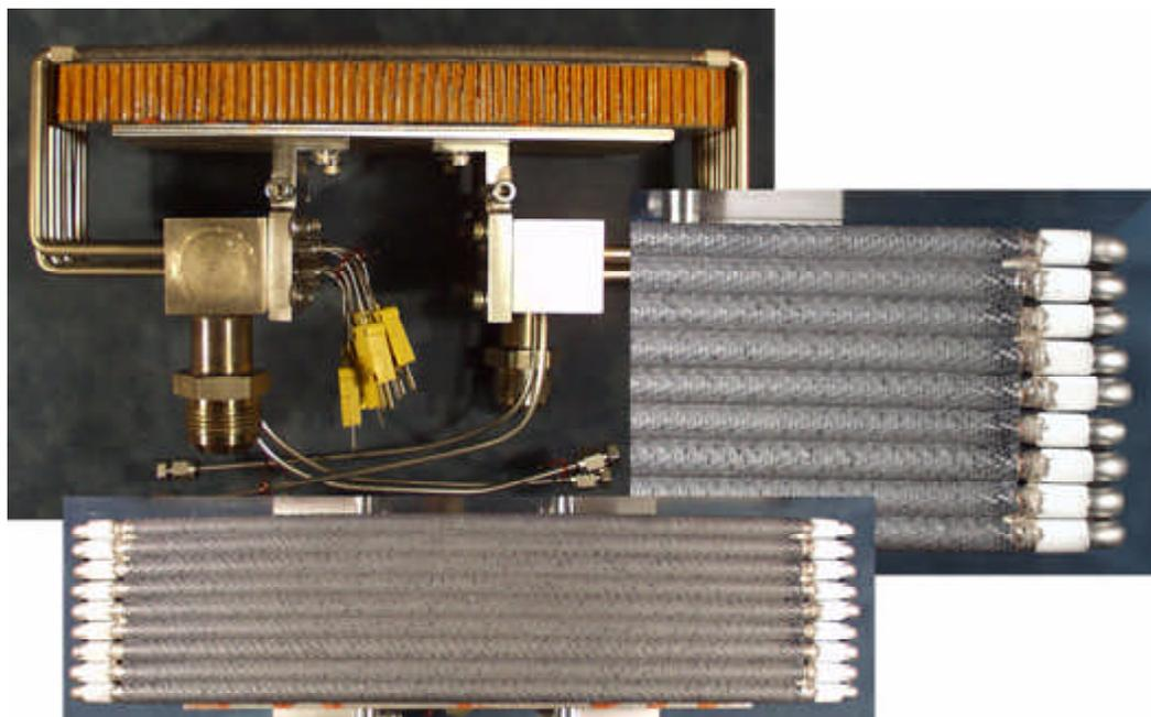
*Cooled CMC panel with woven coolant channels before test firing.*
