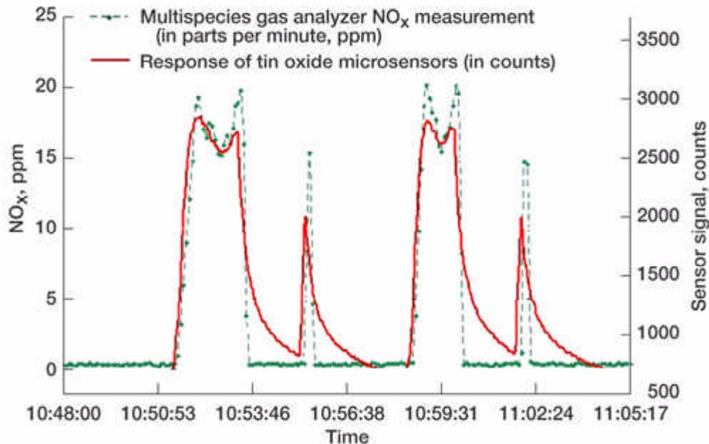
*Comparison of the NO<sub>x</sub> readings measured by the microfabricated sensors and multigas analyzers as the rake is moved across the engine exhaust outlet.*
