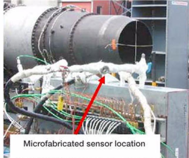
*Microfabricated emissions sensors. Left: The rake sampling system at the outlet of the JT-12 jet engine. Right: Location of the sensors in the flow stream of the rake. The high-temperature operational capability of the sensors allow placement significantly closer to the engine outlet than traditional equipment.*
