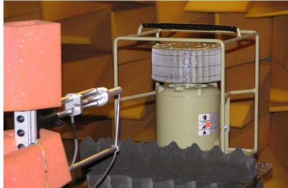
Figure 2. Centrifugal Sound Source and Reference/ Test Microphone
