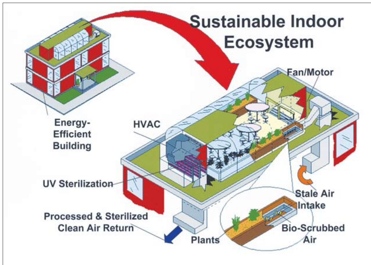
Wolverton Environmental Services Inc. designed this sustainable ecosystem to show how a building's circulation system and a rooftop garden could work in tandem to clean indoor air.
