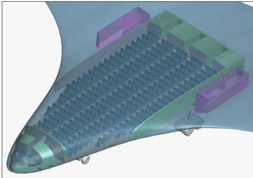
Figure 5. Sample 335-passenger layout for volumetric sanity check.
