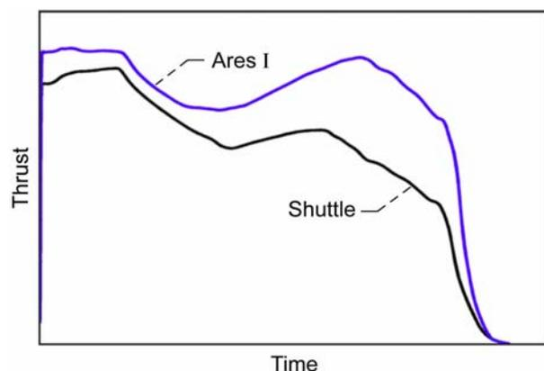
Figure 2.—Thrust trace comparison: Shuttle versus Ares I.
