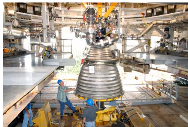
Figure 3.—Powerpack 1-A during test stand installation at SSC.
