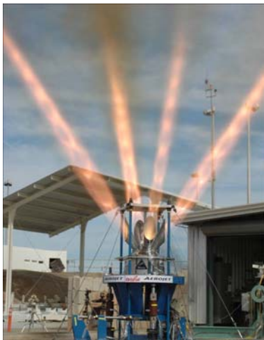
Figure 7.—Orion launch abort system jettison motor test.
