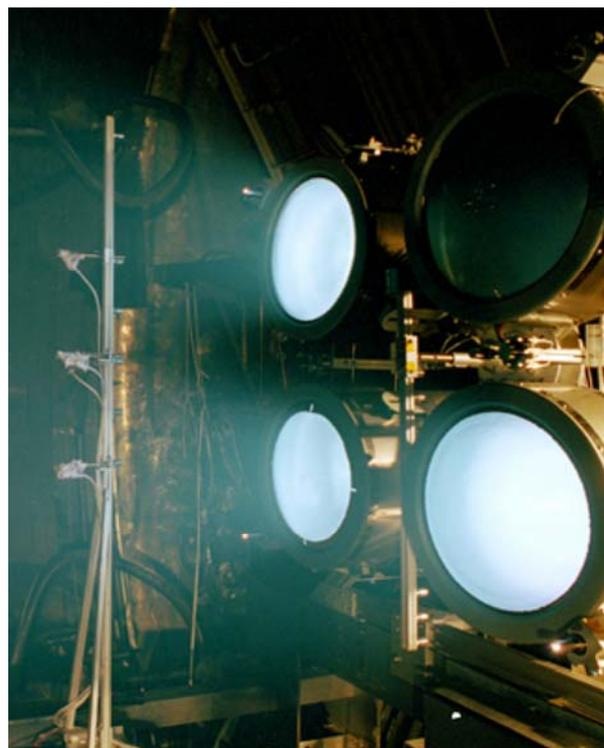
Figure 11.—NEXT multithruster array test.
