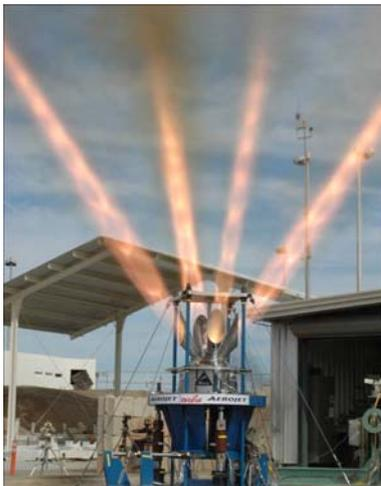
Figure 7.—Orion launch abort system jettison motor test.
