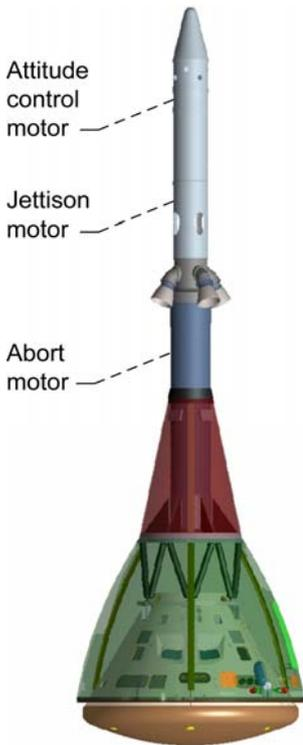
Figure 6.—Launch abort system production configuration.
