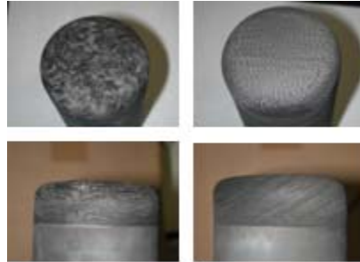
Figure 8: Carbon-phenolic after testing
